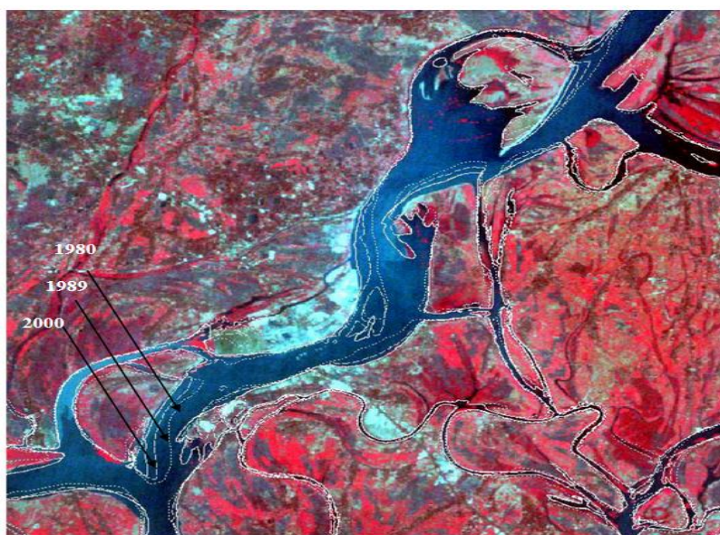
Figure 5.4.8 (c): Bank lines from 1980, 1989 and 2000 superimposed on satellite images from 2010. Area covers from downstream of Meghna Ferry Ghat to upstream of Baiddyar Bazar
